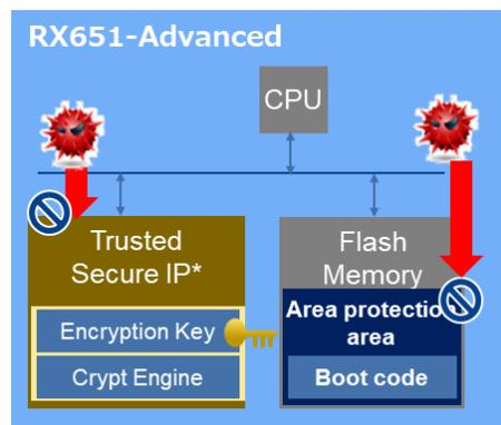
**Figure 2:** Root of Trust realized by Trusted Secure IP and area protection
