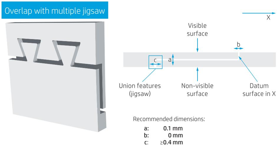
Figure 11: Overlap with multiple jigsaw features: Design recommendations
