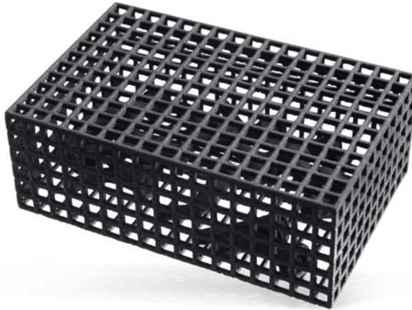
*Figure 7. Cage printed with small parts inside*
