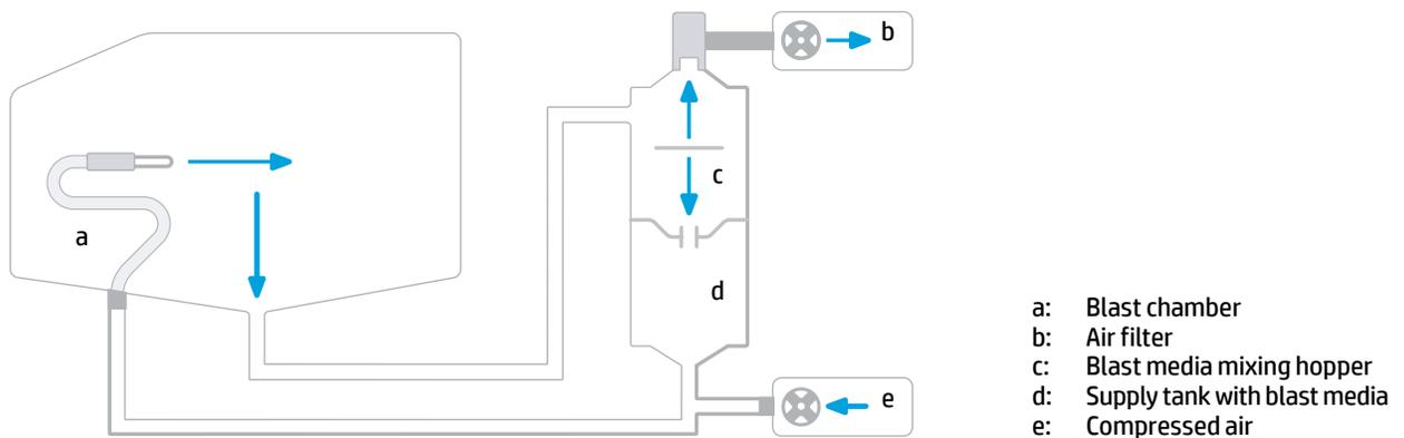
Figure 3. Functional diagram of a bead blaster
