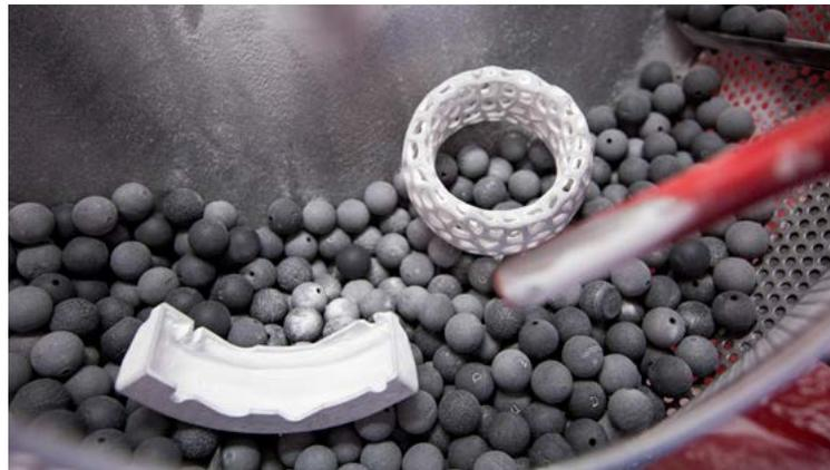
*Figure 4. Automatic bead blaster*
